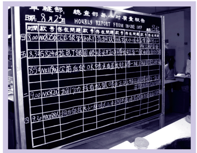
Output data recorded and displayed on the factory floor
